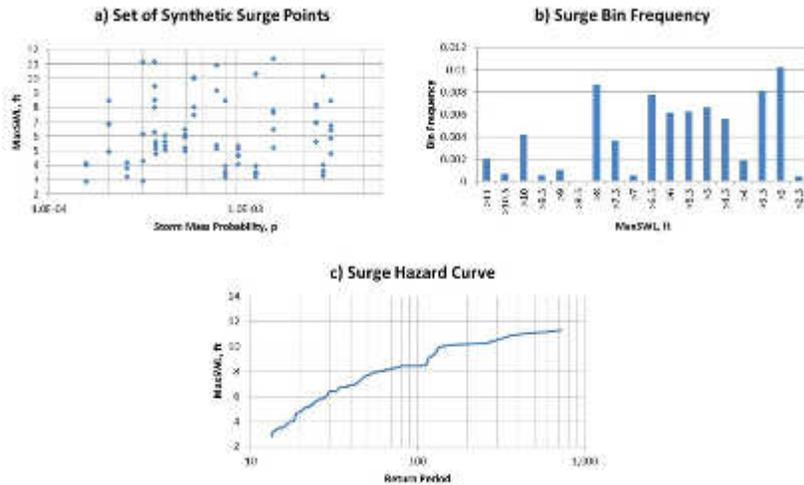
**Figure 6 Construction of a Surge Hazard Curve from JPM Results**
