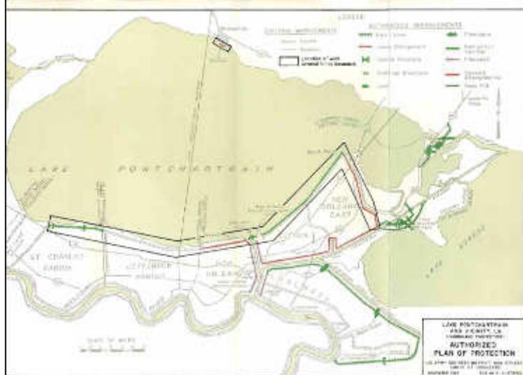
**Figure 2. Barrier Plan for Protecting the New Orleans East-Bank
